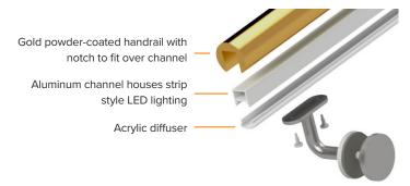
Aluminum, powder-coated handrails with an aluminum channel inset house the strip style LED lighting and conceal wiring. An additional acrylic diffuser was positioned on the underside of the handrail to achieve the desired look of continuous lighting.
