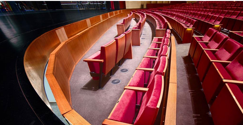
Minimalist in style but sturdy in design features hard panel skirting around the perimeter and acoustical sound dampening on the underside.
