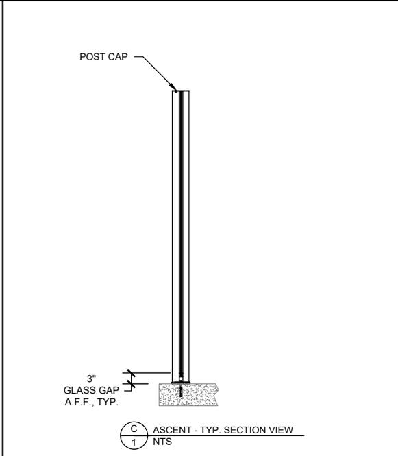
†MAX POST SPACING, MAX GLASS HEIGHT, AND ANCHORAGE VARY WITH PROJECT SPECIFICATIONS. CONTACT TREX COMMERCIAL PRODUCTS FOR DETAILS.
