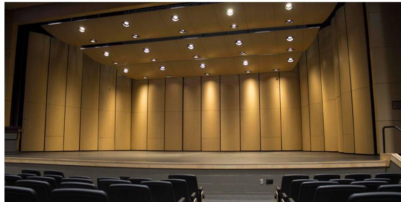
The customizable system includes seven acoustical towers and three ceiling rows.
