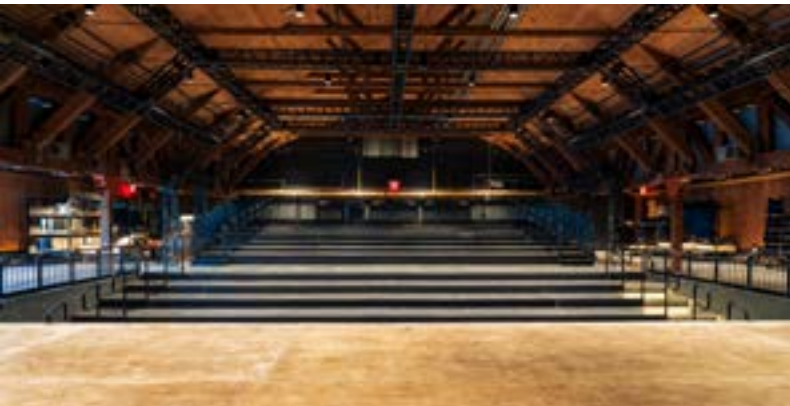
A tailored mix of 3x3, 3x6 and custom platform sizes were used to build seating rows that extend upstage/downstage.
